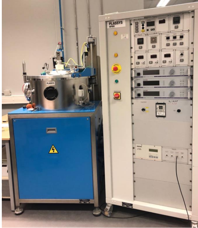
Figure 3.2 RF magnetron sputtering system of Plassys.
