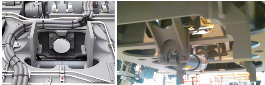
Figure 2.9: Left picture. Pivot hollow on a FLEXX Compact extremity motor bogie for a R2N trainset. The longitudinal bump stop is visible in the middle. Lateral bump stops are attached to the car pivot, which is inserted in the hollow space and links both of the abutting carbodies. Right picture. Lateral motion of the secondary suspension is damped by a dashpot placed under the bogie frame, attached to the carbody pivot. On the upper right corner, barely visible, one of the anti-roll bars. Self-owned picture.
