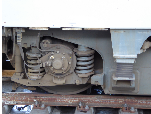
Figure 2.4: Primary coil springs and secondary stack-layered rubber-metal spring on SNCF engine BB 7296. The axlebox traverse is linked to the bogie frame by a traction rod on its right side. Self-owned picture.
