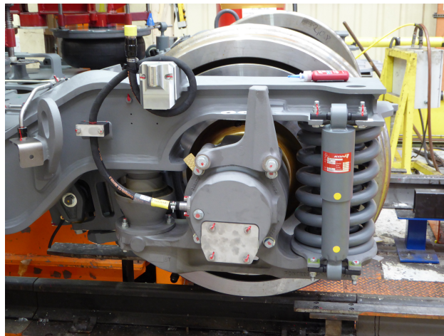
Figure 2.7: Primary suspension on a FLEXX Compact trailer Jakob bogie for a R2N trainset. The primary suspension consists in an outer coil spring on the right of the axlebox, an inner rubber spring on the left of the axlebox, a hydraulic damper parallel to the coil spring and a primary rubber bump stop on top of the axlebox (hidden from the view). Self-owned picture.
