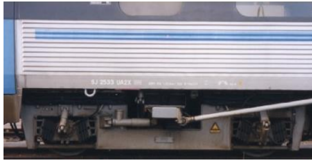
Figure 2.5: The axleboxes are framed by two stack-layered rubber-metal chevrons on each side. Image by https://www.feckin-mad.co.uk/forum/viewtopic.php?t=2608 .
