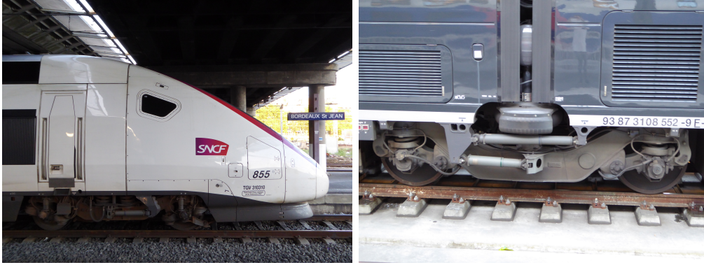
Figure 2.1: TGV bogies (Alstom). The left image is a motor bogie, fitted with rubber-to-metal primary springs and secondary coil springs. On the right, a trailer Jakobs bogie between two cars, with rubber-to-metal primary springs and secondary air spring suspension. Self-owned picture.
