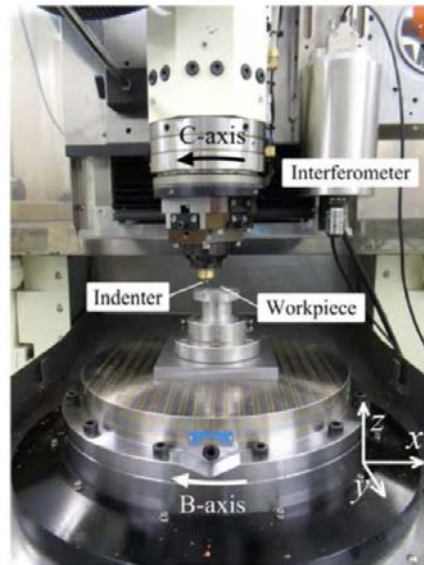
Fig. 38 Single-grit test setup used by Wang et al. [88].
