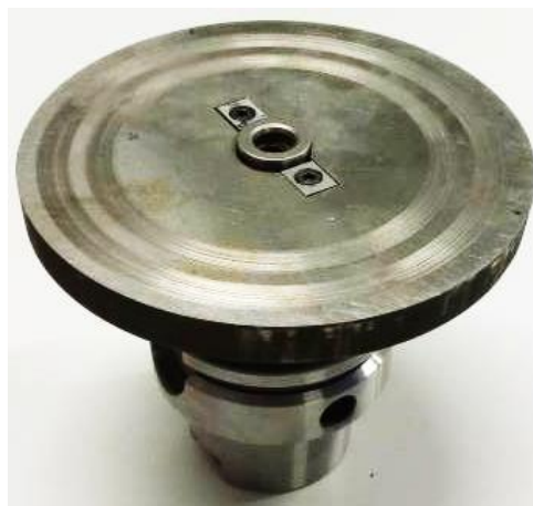
Fig. 103 The Inconel 718 disk fixed on the HSK chuck used for the LST.
