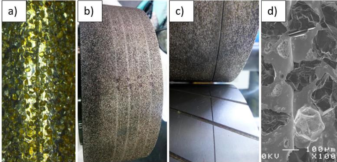
Fig. 71 a) A macroscope picture of a groove on an EP CBN wheel. b) An EP CBN wheel with four grooves on its surface. c) On the top, an EP CBN grinding wheel with a groove on its surface, on the bottom, the steel body of an EP CBN wheel where the groove reached to the steel body. d) A SEM picture of a groove on an EP CBN grinding wheel.
