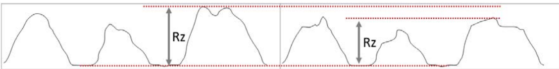
Fig. 90 A hypothetical wheel profile after and before conditioning. The profile on the right has lower R_a and R_z .
