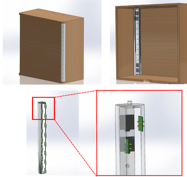
Figure A.2 – Simplified truck model with a movable cylinder equipped with 20 micro-blowers. Figures obtained from Minelli (2017)
