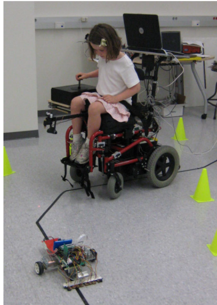
Figure 2.17: Robotic wheelchair guided the children to learn driving skills using force feedback joystick [39].
